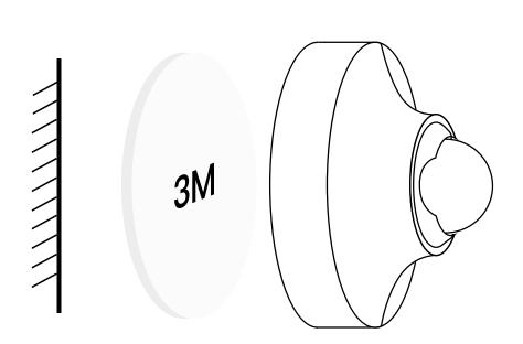
Tighten the camera, and clamp the snap. Adjusts the camera angle according to the display of the mobile phone
